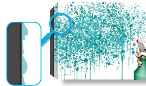
Inconsistent coverage with drips and runs
